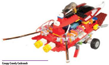
This super smart cockroach easily navigates through any environment using bend sensors and light triggers.
